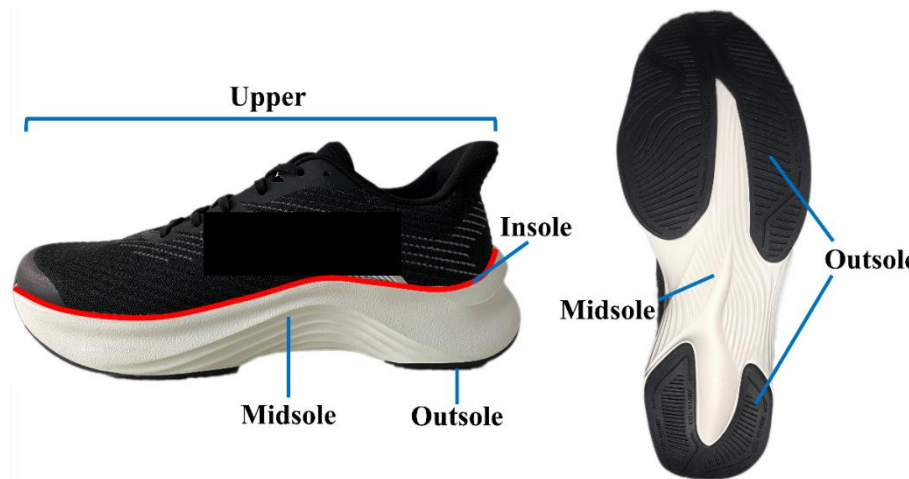
Figure 6 The basic structure of a running shoe
